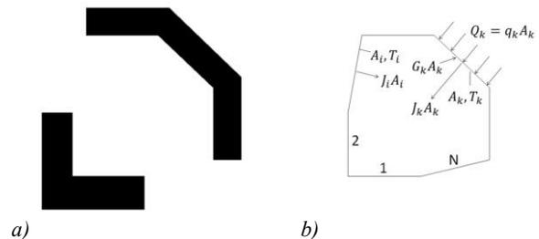
Figure 1: Building envelope in urban environment could be treated as an enclosure of  $N$  surface areas each of uniform temperature  $T_i$  (a) building blocks shown in plan; and (b) radiative transfer within enclosure formed by building envelope.
