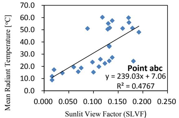
Figure 3: Scatter plot for Mean Radiant Temperature against Sunlit View Factor using 5-min mean values for the three measurement points a, b, and c.
